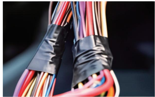
Wire and cable strapping
